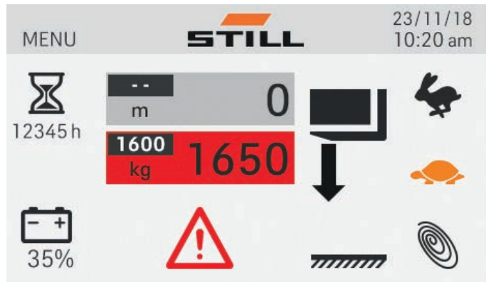
Safe storage and retrieval thanks to Dynamic Load Control, the residual load capacity warning system
