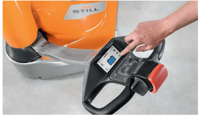
Everything in view, all the time: optional touch display with a range of language-independent symbols shows all important functions at a glance
