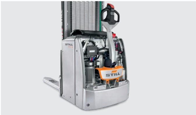
Low-maintenance components and easy service access
