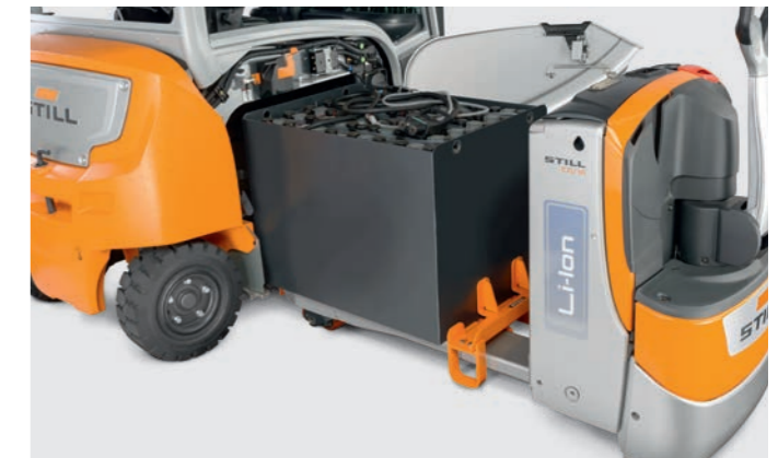
Battery change with electric pallet truck
