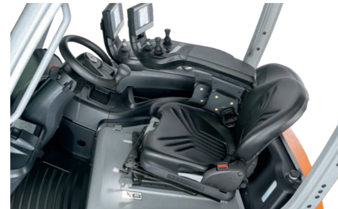
Swivel seat for comfortable reversing
