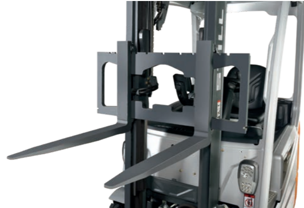
Optimal view of fork tips when loading HGVs
