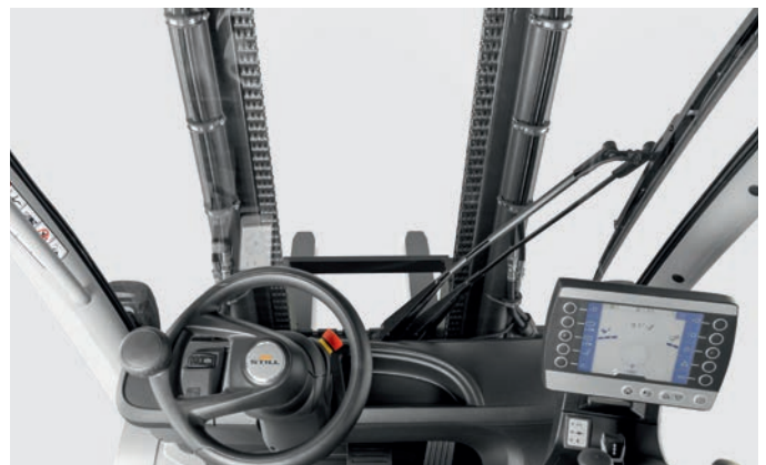
Telescopic mast for outstanding visibility ahead
