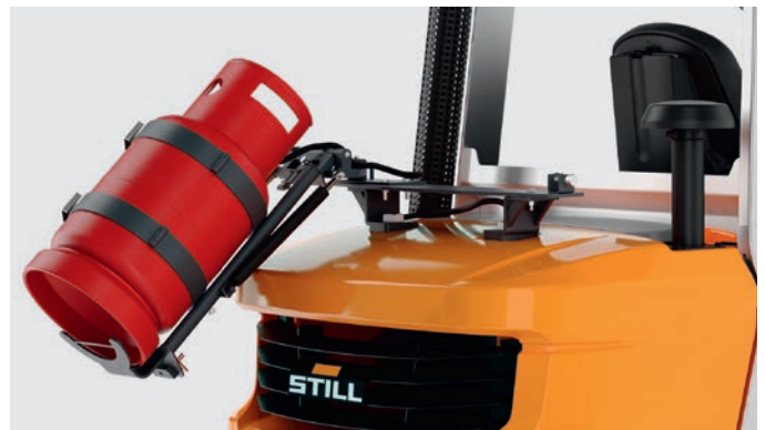
Ergonomic gas cylinder exchange: Swivelling fold-out holders make changing the LPG cylinder quick and easy
