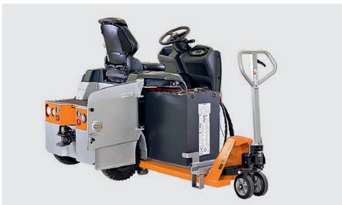
STILL's proven lateral battery change ensures optimum vehicle availability and ergonomics
